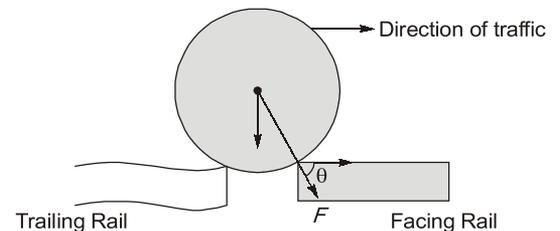
**(c) Dragging Theory:** Due to friction force between wheel & rail a drag force generate opposite to movement of train, resulting in creep.
